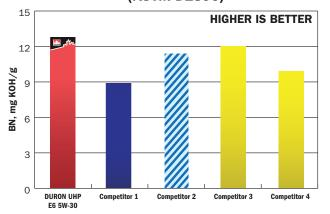
BN is a measure of the oil's potential ability to neutralize harmful acids formed during the combustion process. Counteracting harmful acids helps to mitigate potential corrosion caused by the acids.
